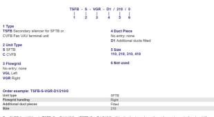
For CVFB fan VAV unit, TSFB-C-..-D1/110/0 or TSFB-C...-D1/210/0 will be the basic code as the unit requries only the size 110 or 210 attenuator with D1 additional ducts
