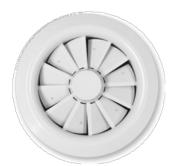
VDL swirl diffusers are suitable for large volume flow rate ranges and can be adjusted mechanically or manually. Blade adjustment allows for optimum ventilation (purging) of the occupied zone while high comfort requirements are met at the same time.
