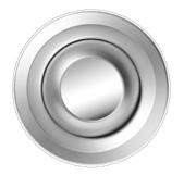
The adjustable TJN jet nozzles are made of high-grade polymer and allow for adapting the supply air flow to different conditions. The enhanced jet nozzles are acoustically optimised and more energy-efficient than similiar products since the actuator is fitted on the outside and does not lead to any additional pressure drop. 20 – 1,000 l/s
