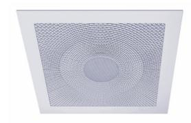
PROCONDIF Profile Controlled Diffusion These diffusers are also an excellent solution for providing supply air from above to sensitive areas in labs, creating a displacement flow in the occupied zone. 280– 600 m³/h 78 – 167 l/s 600 x 600, 625 x 625 mm
