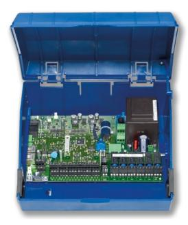
EASYLAB control components for room pressure control in sensitive areas.
