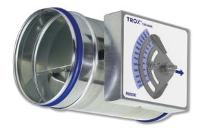
CAV controller RN – for supply air and extract air systems, easy volume flow rate setting without any tools V: 11 – 1,400 l/s V: 40 – 5040 m³/h  $\Delta$ p: 50 – 1000 Pa Ø 80 – 400 mm Closed blade air leakage to EN 1751, class 4 Casing air leakage to EN 1751, class C
