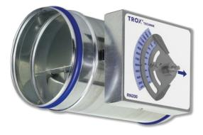
CAV controller RN – for supply air and extract air systems, easy volume flow rate setting without any tools V: 11 – 1,400 l/s V: 40 – 5040 m<sup>3</sup>/h  $\Delta$ p: 50 – 1000 Pa Ø 80 – 400 mm Closed blade air leakage to EN 1751, class 4 Casing air leakage to EN 1751, class C
