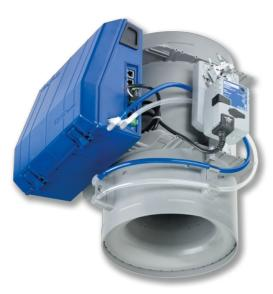
VAV terminal unit TVLK, made of plastic, for lab extract air systems, for the removal of aggressive media V: 30 - 515 l/s V: 108 - 1854 m<sup>3</sup>/h ∆p: 5 – 1000 Pa Ø 250 mm Closed blade air leakage to EN 1751, class 4 Casing air leakage to EN 1751, class C
