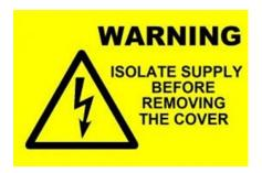
Only skilled qualified electricians are allowed to open the controls access panel. Ensure that the electrical supply is isolated and verify that no voltage is present on any mains circuit before you open the cover to access the terminal connections.
