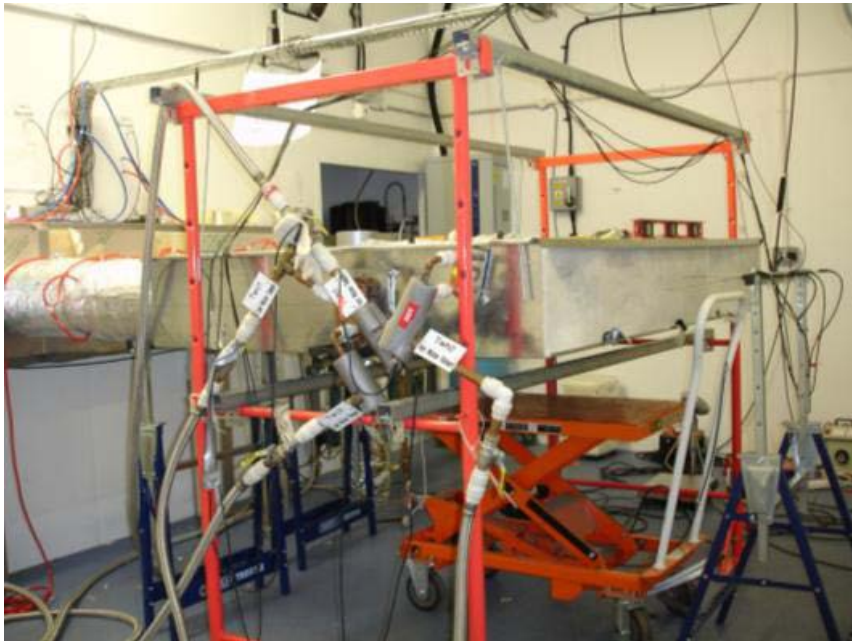
Example of a FCU in TROX'S BSRIA certified Thermal test chamber.
