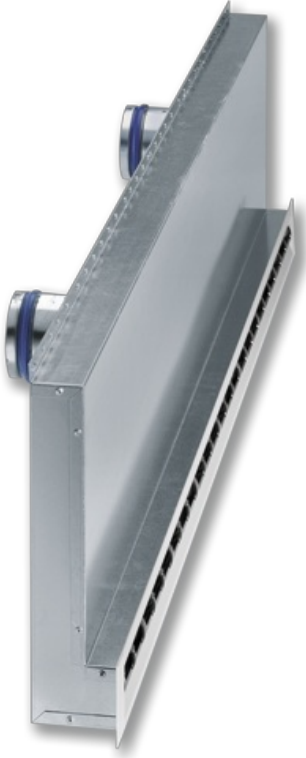
Combination diffusers of Type VSD50-1-LT 14 - 55 l/s 50 - 200 m 3 /h L: 550 und 1.175 mm B: 70 mm With integral acoustic lining
