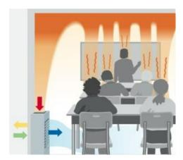
Classrooms place high demands on supply and extract ventilation. They are sometimes used extensively with up to 30 people. A fresh air flow rate from 15 to 20 m3/h is usually assumed for each person. This results in an overall volume flow rate from 300 to 600 m3/h per classroom.
