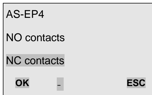
Figure 6.10.5: Setting of NO or NC contacts
