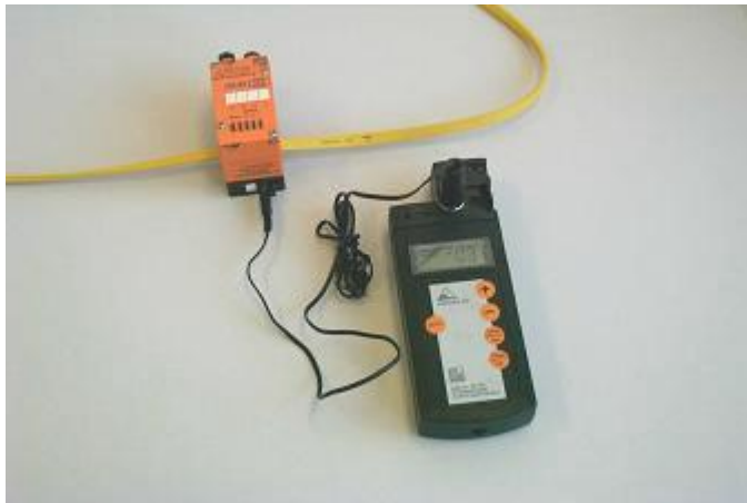
Figure 7.3.1: Addressing of an AS-i module via the addressing plug
