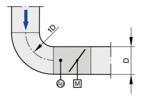
A bend with a centre line curvature radius of at least 1D – without an additional straight duct section upstream of the VAV terminal unit – has only a negligible effect on the volume flow rate accuracy.
