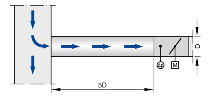
A junction causes strong turbulence. The stated volume flow rate accuracy  $\Delta V$  can only be achieved with a straight duct section of at least 5D upstream. Shorter upstream sections require a perforated plate in the branch and before the VAV terminal unit. If there is no straight upstream section at all, the control will not be stable, even with a perforated plate.
