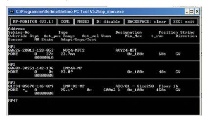
PC-Tool with monitor function/ connection: ZK2-GEN to MP client
