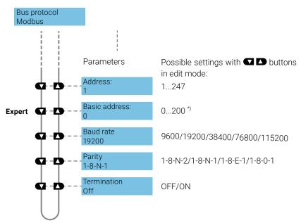
$^{\star}$ )The setting of the base address is also taken into account for the BACnet MS/TP address.
