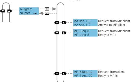
If it is determined that telegrams are being erroneously conveyed, then this will be indicated visually with a "!" as a mark of mistrust.
