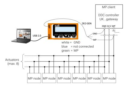
PC tool with monitor function/ connection: tool socket with ZK6-GEN, ZK4-GEN
