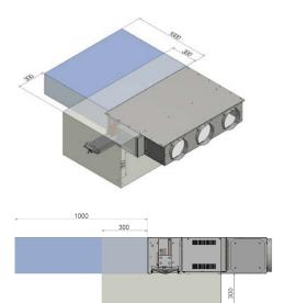
For correct air entry conditions, a minimum of 1000mm should be provided on the inlet of the fancoil to allow free passage of air into the unit. Failure to observe this access will restrict airflow into the fancoil increasing noise level and decreasing electrical efficiency.
