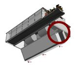
5. To re-install the fan access panel, carefully offer up the access panel hinge flange into each notch on the fancoil casing. Once engaged, slide the access panel towards the discharge plenum (away from the drip tray) and rotate up to its closed position. Secure the access hatch in place using the M5x12 POZI PAN HD screws and tighten securely.
