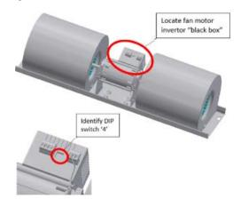
Depending on the control configuration, DIP '4' will be set to **ON** or **OFF**
