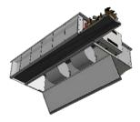
To fully remove the fan access panel, pull the panel towards the drip tray until the hinge return reaches the notch within each side of the fancoil casing. Manoeuvre each hinge flange out of the notch and store access panel safely at floor level to avoid injury or damage.
