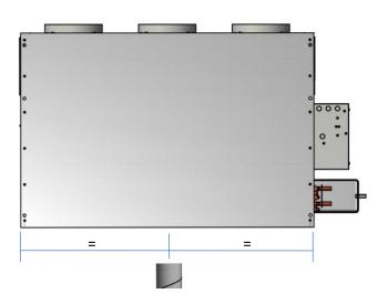
The discharge velocity from the fresh air duct should be maintained at  $\leq$  2.0 m/s.
