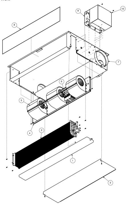
Fig 1: Waterside fancoil unit
