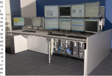
heat exchangers for the highest levels of resilience. In addition, for built in redundancy, each unit contains two power supplies and two fans so that in the event that one fan fails, the other has the capacity to provide 75% of the load which would be adequate for most situations until the maintenance team arrives.
